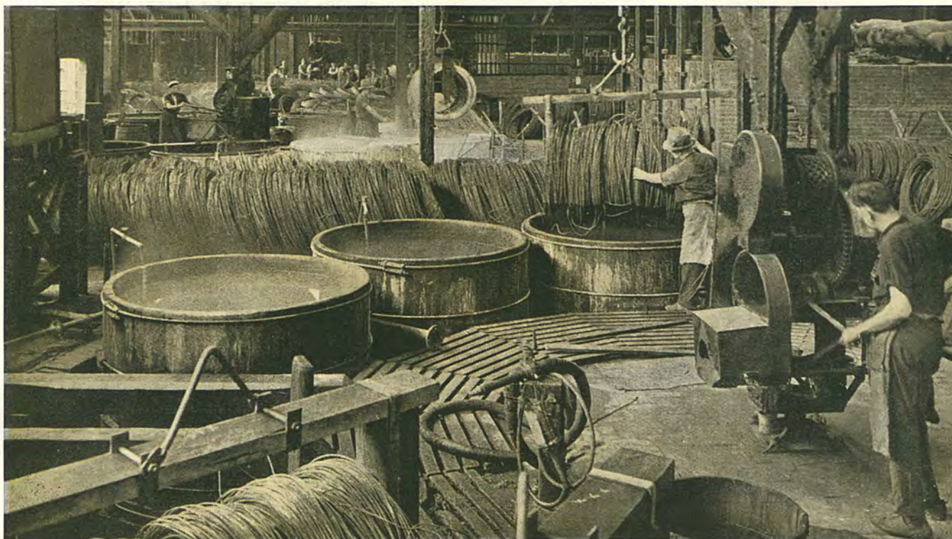
CLEANING DEPARTMENT WHERE RODS ARE PREPARED FOR THE WIRE DRAWING OPERATION.
