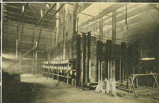
Top, right: Blast Furnaces, bottom floor, running off slag. Bottom, right: Zinc Distillation Plant, Prolongs in position.
