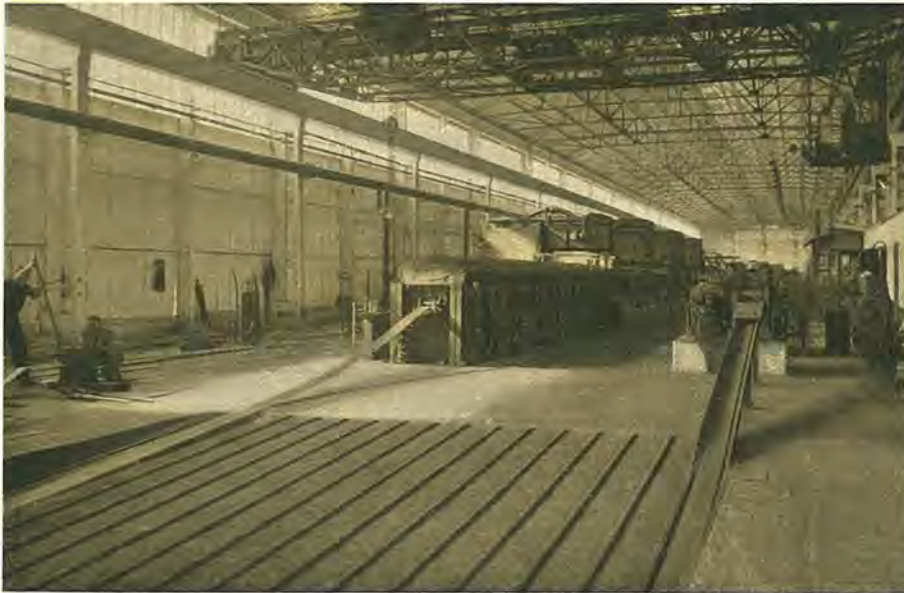
COLD END OF FURNACE With skelp entering and showing ends of skelp loop.
