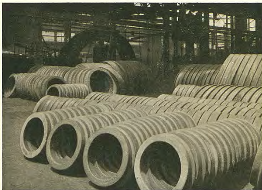
TYRE MILL STOCK YARD. TYRES AWAITING MACHINING.
