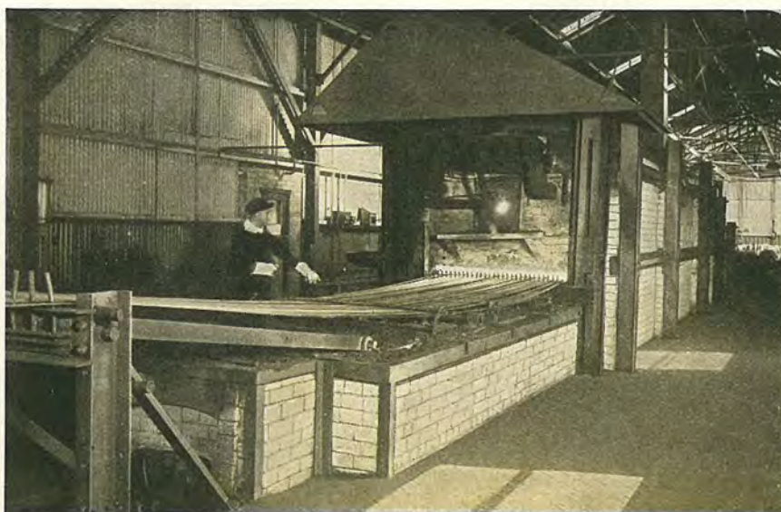
30 WIRE PATENTING FURNACE. For Heat Treatment of Rope and Spring Wires.
