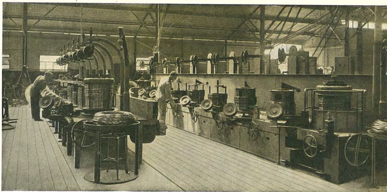
HIGH SPEED CONTINUOUS WIRE DRAWING MACHINES.
